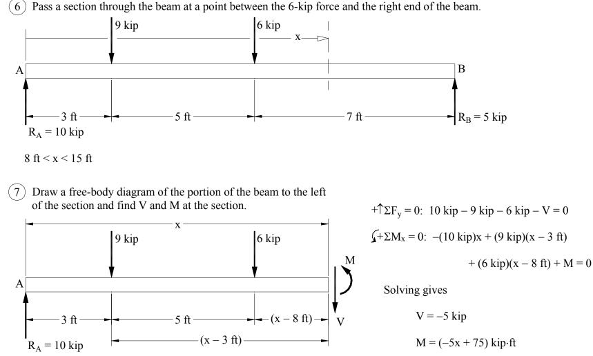
Pass a section through the beam at a point between the 6-kip force and the right end of the beam.
