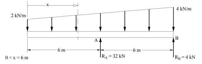
8 Draw a free-body diagram of the portion of the beam to the left of the section and solve for V and M.
