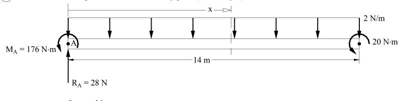
3) Pass a section through the beam at an arbitrary point (located by x) (
