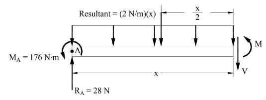
+↑ $\Sigma F_y = 0$ : 28 N - 2x - V = 0  $\int +\Sigma M_x = 0$ : 176 N·m - 28x +  $(\frac{x}{2})(2 \text{ N/m})(x) + M = 0$
