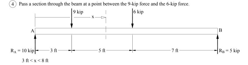
5) Draw a free-body diagram of the portion of the beam to the left of the section and find V and M at the section.
