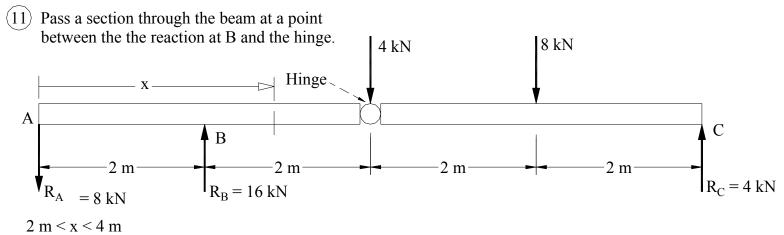
(12) Draw a free-body diagram of the portion of the beam to the left of the section and find V and M at the section.
