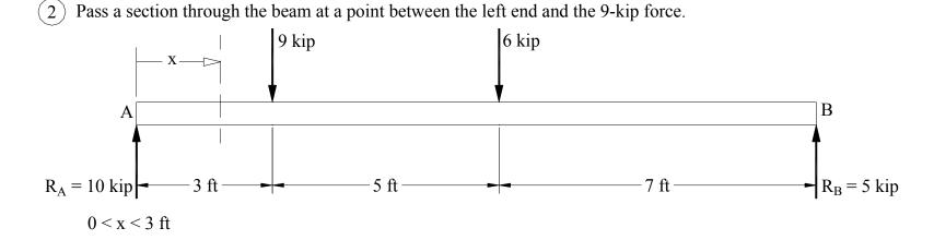
3 Draw a free-body diagram of the portion of the beam to the left of the section and find V and M at the section.
