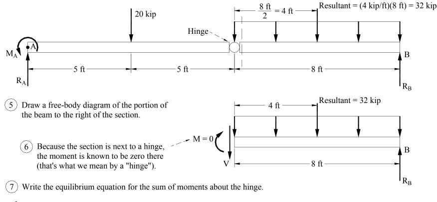
$$\int + \Sigma M_{\text{hinge}} = 0: -(32 \text{ kip})(4 \text{ ft}) + R_{\text{B}}(8 \text{ ft}) = 0$$
