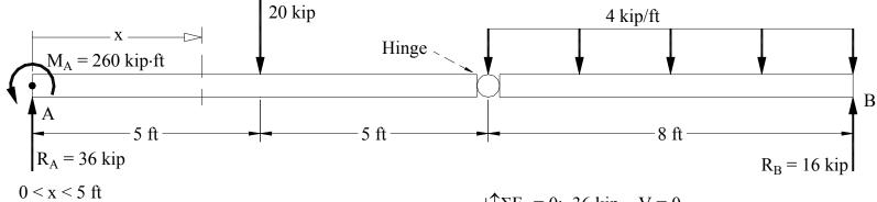
(1) Draw a free-body diagram of the portion of the beam to the left of the section and find V and M at the section.
