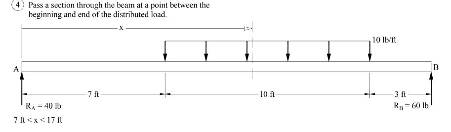
5 Draw a free-body diagram of the portion of the beam to the left of the section and solve for V and M at the section.
