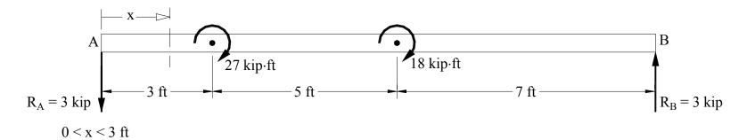
(3) Draw a free-body diagram of the portion of the beam to the left of the section and find V and M at the section.
