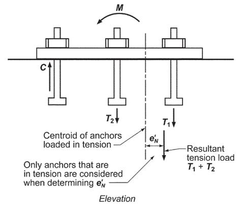
**Fig. R17.4.2.4**—Definition of  $e'_N$  for a group of anchors.
