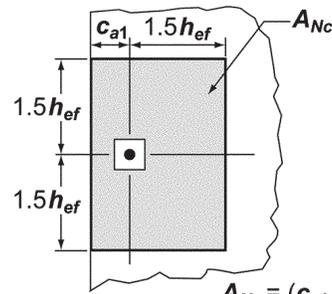
$$A_{Nc} = (c_{a1} + 1.5h_{ef})(2 \times 1.5h_{ef})$$
