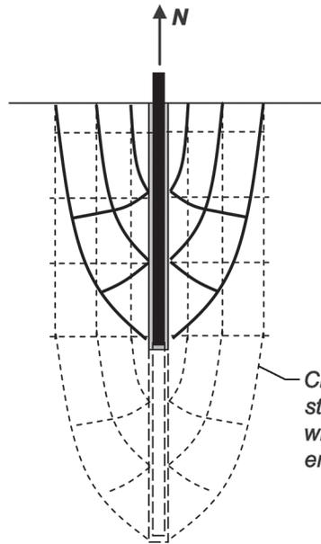
Section through anchor showing principal stress trajectories
