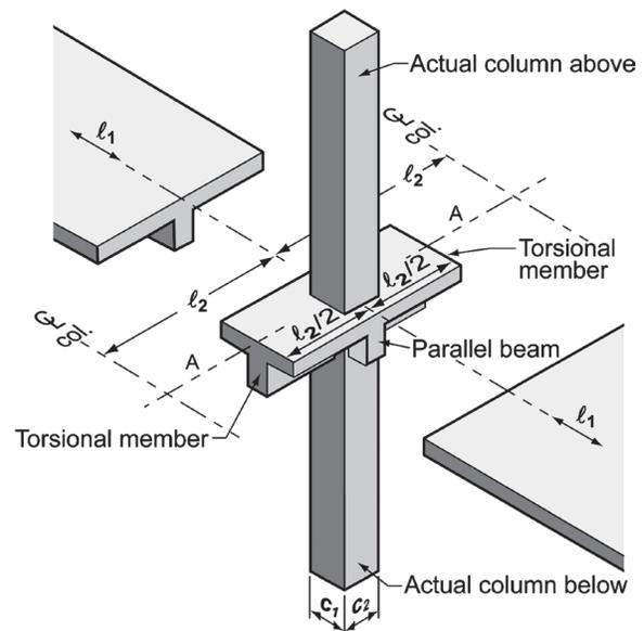
**Fig. R8.11.4**—Equivalent column (column plus torsional members).
