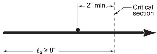
**Fig. R25.4.6.3**—Development of welded deformed wire reinforcement.
