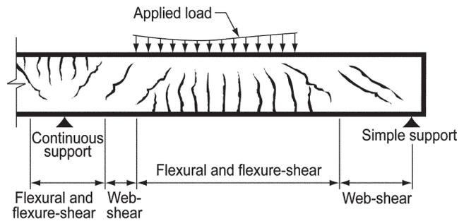
Fig. R22.5.8.3—Types of cracking in concrete beams.
