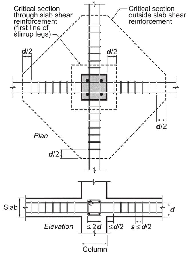
**Fig.R8.7.6d**—Arrangement of stirrup shear reinforcement, interior column.
