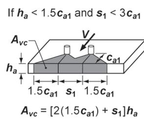
**Case 1:** One assumption of the distribution of forces indicates that half of the shear force would be critical on the front anchor and the projected area. For the calculation of concrete breakout,  $c_{a1}$  is taken as  $c_{a1,1}$ .
