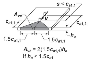
**Case 3:** Where  $s < c_{a1,1}$ , apply the entire shear load  $V$  to the front anchor. This case does not apply for anchors welded to a common plate. For the calculation of concrete breakout,  $c_{a1}$  is taken as  $c_{a1,1}$ .
