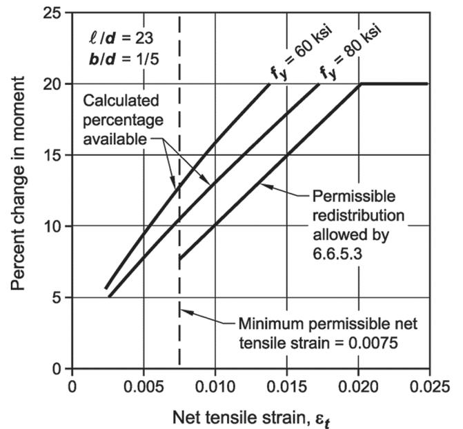
Fig. R6.6.5—Permissible redistribution of moments for minimum rotation capacity.
