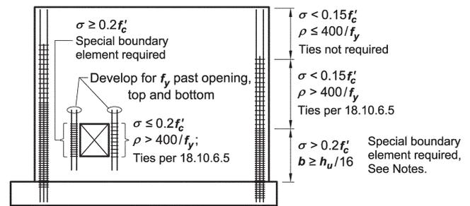
Notes: Requirement for special boundary element is triggered if maximum extreme fiber compressive stress  $\sigma \geq 0.2f'_c$ . Once triggered, the special boundary element extends until  $\sigma < 0.15f'_c$ . Since  $h_w/\ell_w \leq 2.0$ , 18.10.6.4(c) does not apply.
