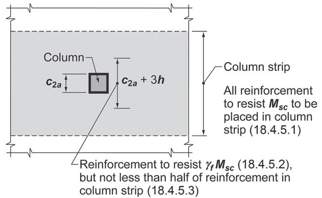
**Note:** Applies to both top and bottom reinforcement
