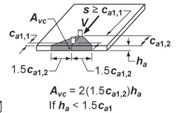
**Case 2:** Another assumption of the distribution of forces indicates that the total shear force would be critical on the rear anchor and its projected area. Only this assumption needs to be considered when anchors are welded to a common plate independent of  $s$ . For the calculation of concrete breakout,  $c_{a1}$  is taken as  $c_{a1,2}$ .
