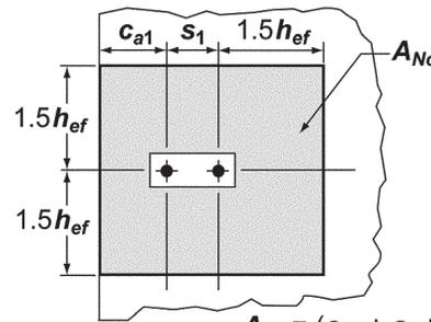
$$A_{Nc} = (c_{a1} + s_1 + 1.5h_{ef})(2 \times 1.5h_{ef})$$
