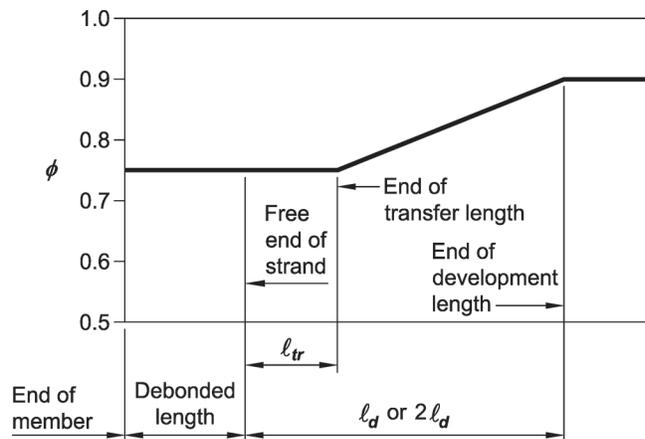
Note: The location of the end of development length depends on the calculated stresses in the extreme concrete fiber of the precompressed tension zone under service loads.
